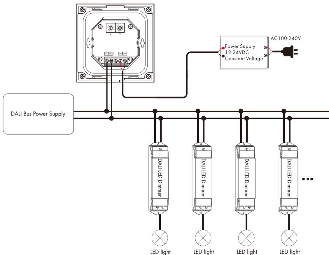
Note: It is recommended to use a 24VDC power supply for the touch panel DALI master to reduce the load on the DALI bus power supply.
