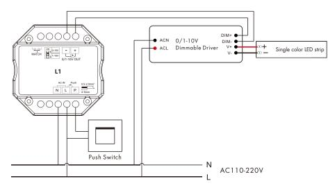
Note: We recommend the number of LED drivers connected to 0/1-10V dimmer does not exceed 50 pieces, the maximum length of the wires from dimmer to LED driver should be no more than 50 meters.
