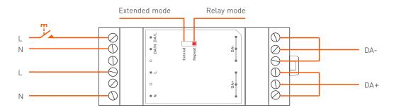
Push DIM (For extended mode only) 0-100% dimming range. Short press to turn on /off, long press to dim
