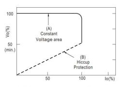
Typical output current normalized by rated current (%)
