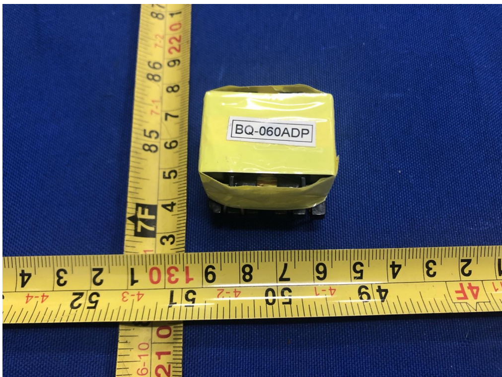
Figure 16. Transformer external view of model BQ-060ADP
