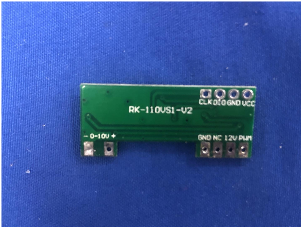
Figure 15. 0-10V Dimming PCB view of model BQ-060ANPC
